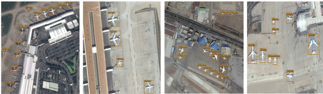
Fig. 5 Detection performance of YOLOX-NR in RSOD dataset aircraft images
