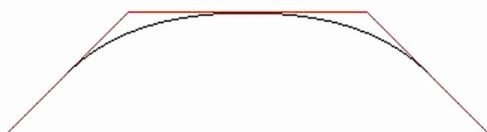
Fig. 1 The uniform quadratic B-Spline Curve
